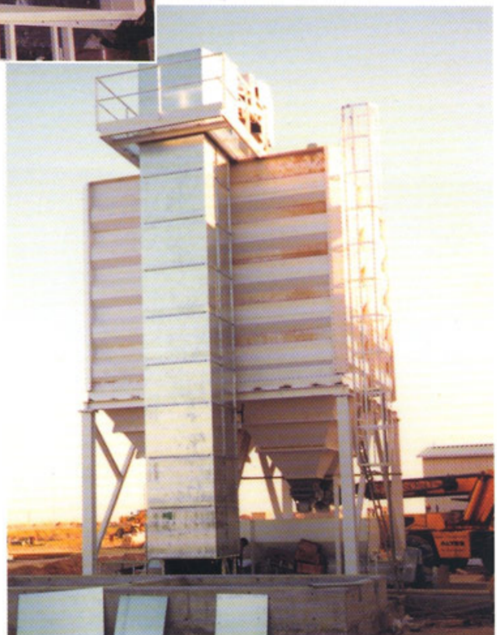
TEB for extraction from 33 m. profundity of excavation in the collector tunnel, with hopper and truck loading system.
