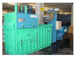
The PET-perforator "PF 800" can also be used as a pre-compressor of a small baling press.
