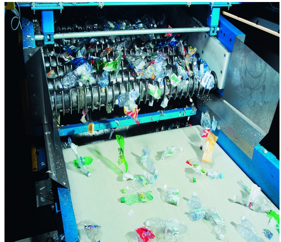
... with the BOREMA disk and acceleration screen 100-160 for top sorting quality and capacity.
