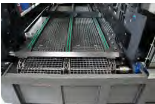
Oil collection tray with accessible grating segments, incl. level monitoring
