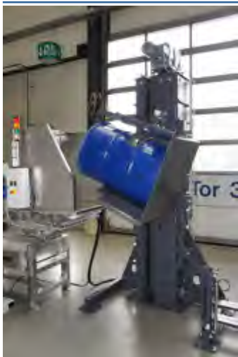
The lift-tipper feeds the full barrel into the hopper of the manual sorting table
