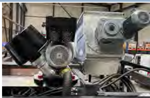
Fan for cleaning the pressed oil filter
