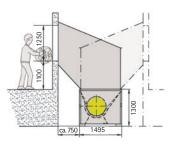
feeding via wall-connected filling chute
